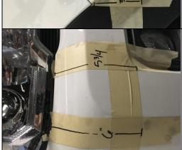
7.) Here you can see the measurements for under the headlight. Measure 6in from the bottom corner of the light and 5 3/4in from the location just under the light as shown. Again the rule of thumb is measure 3 times cut once. You can also follow the line just above the fog light as a reference point of where to cut.
