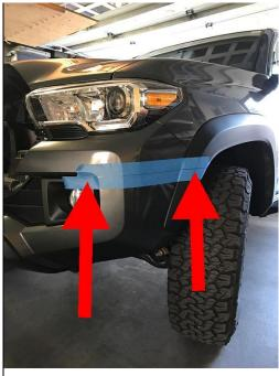
5.) The next step is the cutting of the factory bumper. Be sure to follow the rule of measure 3 times cut once. We tape off the surrounding area for cutting with masking tape. You want to continue the line straight across from under the bumper cut line, shown on the left with the left arrow o. Follow that line across to the fender flare.
