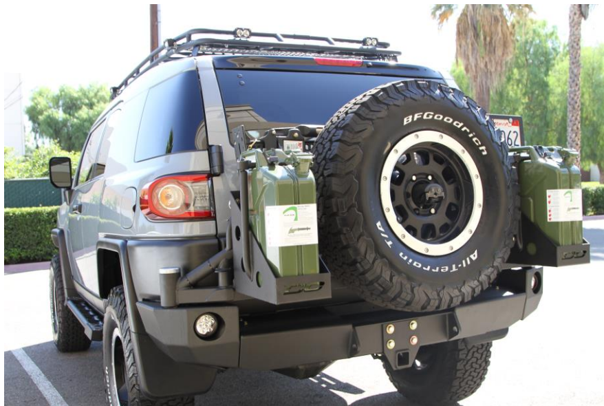
Rear swing out shown with optional Jerry can holders on both sides.
