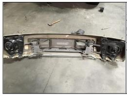
Step 20.) You are now ready to insert the winch plate into the center section of your lower bumper piece. This is the most difficult part of the installation and we recommend taking your time and possibly using someone else to hold the factory bumper while you install the winch plate. (shown with winch installed)
