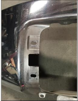
Step 14.) Continued, the bumper should look like this on both sides once the piece has been cut and removed.
