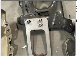
Step 19.) Using the two black bracket pieces and the supplied bumper braces that come with the winch plate. There is a Left and a Right one. They only fit one way. Note in the picture how they go.
