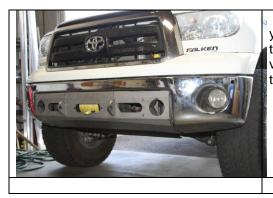
Step 26.) once the lower part of the bumper is reinstalled you can now install the factory fill piece shown as white in the pictures. Reverse steps 1-8 to re-install the top valance piece. If you have any question, please feel free to call so we can walk you through it.
