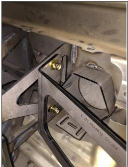
Step 21.) note how brackets mount and go around fog light holes. Snug down the brackets but do not tighten until winch plate is installed on truck.
