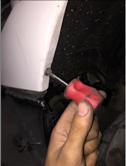
Step 6.) You can use a Philips screwdriver or 10mm socket to remove the other bolt in the fender well.
