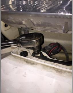
Step 7.) There are also 4 bolts on each side underneath the headlights, these need to be removed and saved for reinstallation.
