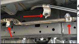
4.) You will then need to remove any bolts that secure the KDSS lines in place as well as your e-brake cable. Do not dis-guard any of it as it gets re-installed.
