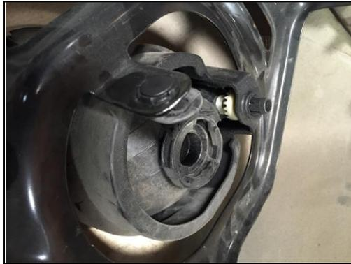
Step 11.) Remove the clip that supports the fog light housing. You can access it from behind the wheel well.
