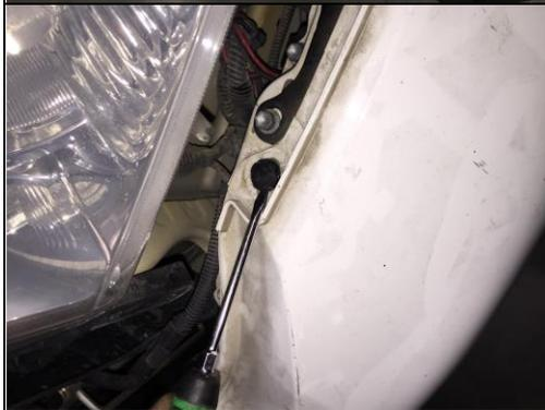
Step 4.) Now you have access to the top plastic bumper valance and assorted plastic clips remove the four plastic clips you now have access to, under the head lights.
