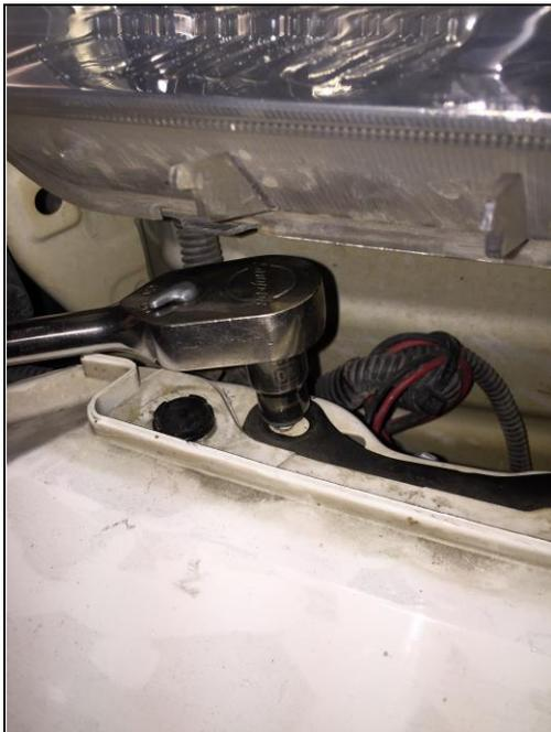
Step 7.) There are also 4 bolts on each side underneath the headlights, these need to be removed and saved for re-installation.
