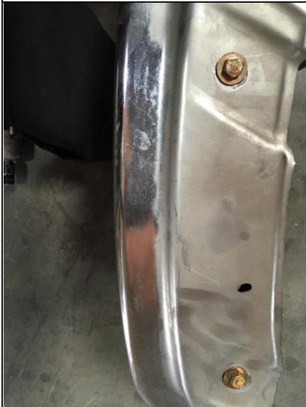
Step 9.) Now that the top piece is removed, you will find 4 bolts on each side on the metal part of the bumper with a total of 4 bolts on top and then an additional 4 on the bottom of the bumper.
