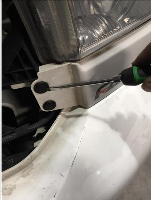
Step 2.) Remove the two black clips on either side on the fill piece under the head lights. Carefully use a small flat head screw driver to pop the rivets out. (DO NOT DISGUARD) You will re-use these clips.
