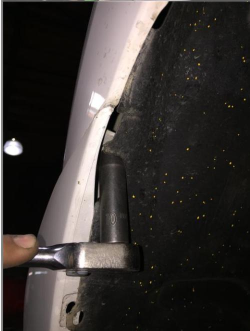
Step 5.) Remove the bolt in the inner fender wheel well. This is a 10mm bolt and can be removed with a ratchet and socket.
