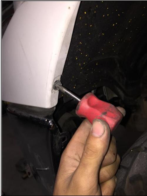
Step 6.) You can use a Philips screw driver or 10mm socket to remove the other bolt in the fender well.
