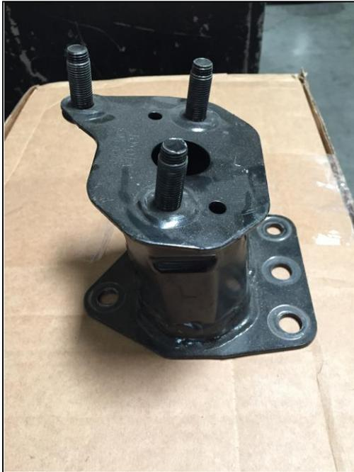
Step 14.) you will also need to remove the steel frame horn from the frame. It has 4 bolts for each one with a total of 8 for both sides. The bolts are 14mm as well and you can use a socket and racket or box end wrench.
