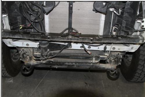
Step 15.) Now that the bash bar and frame horns are removed you have an exposed set of frame rails. .
