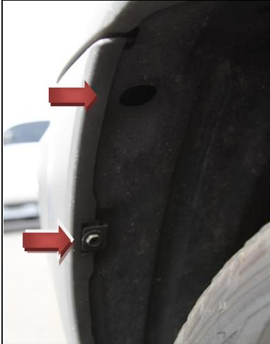
2.) on the out side edge of the stock bumper you will find 12 10mm bolts and screws. They are located in each fender well, under the bumper and under the grill. Remove all these bolts and screws.
