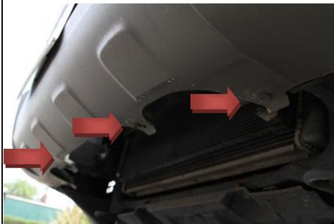
3.) Carefully detach the bumper from each inner fender plastic by gently tugging at the bumper, working your way up and down and alternating from passenger side to driver side.
