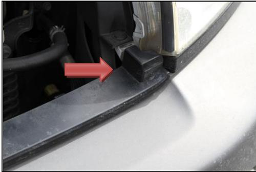
**OPTIONAL:** On 2003-2005 models have a small plastic piece that attaches to the factory bumper. This can be unclipped from the factory bumper and lined up below the grill. It will require drilling two small 1/8in holes in the factory head light mount and re-using some of the factory 10mm screws. This is optional and not required.
